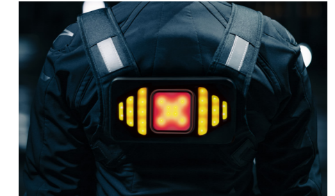
3. Secure the Signalling Unit to the Harness with the Scratch Bands and place the harness on your back
